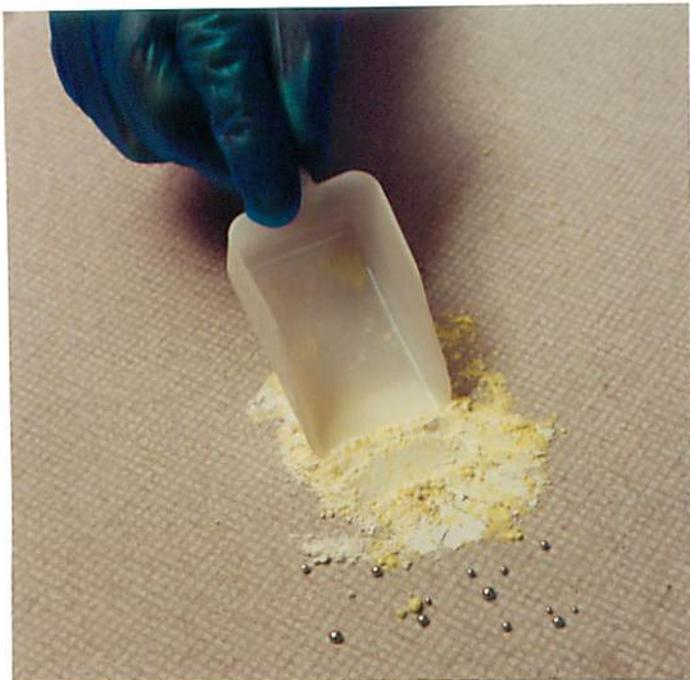
6) Using the scoop, mix the powders with the spilt mercury
