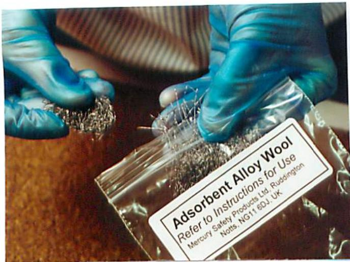
5) Using the Alloy Wool like a cotton wool bud, dab it onto the remaining mercury. Allow the wool to remain in contact with the mercury. Do not press hard or you may force the mercury into the pile of the fabric.
