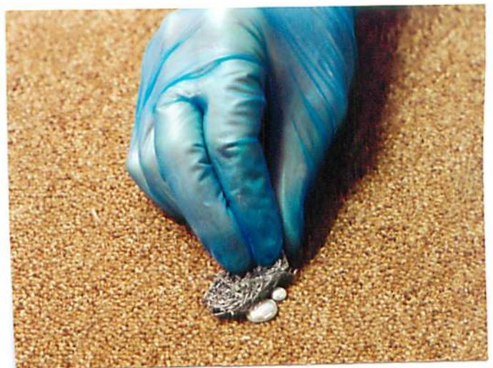
6) You will see the mercury filling the gaps between the metal strands as it forms an amalgam. The Alloy Wool 'bud' will hold the mercury.
